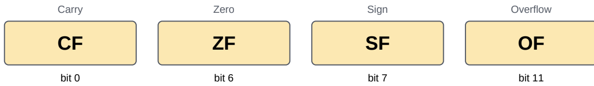
Figure 2.3: The four flags used by conditional jumps.
